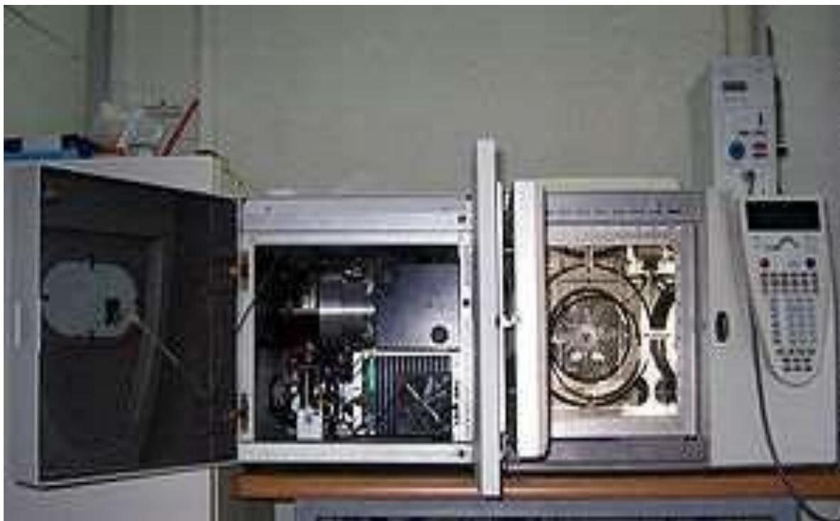
The insides of the GC-MS, with the column of the gas chromatograph in the oven on the right.
